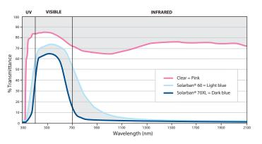
As this chart demonstrates, compared to clear glass and another leading solar control low-e glass, Solarban 70XL glass dramatically reduces the amount of infrared energy (heat) that enters your home while still providing high levels of visible light transmittance (sunlight).
